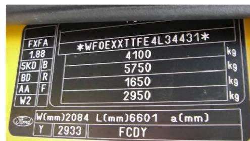
The relevant weight is always the **second biggest weight on the plate** – in this case 4100kg. If you are unsure, ask the minibus owner. This plate is on
